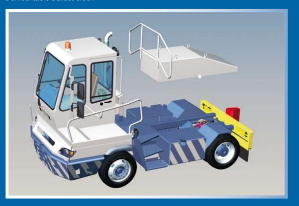
Special drawbar coupling and camera system to inform the driver
