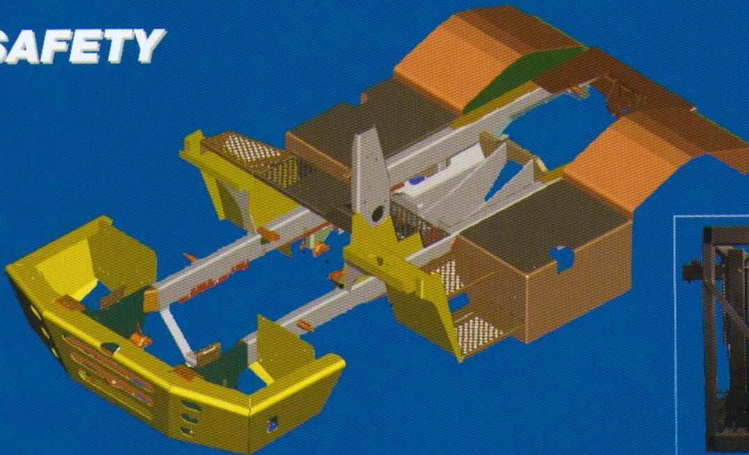
The fully welded chassis frame provides a perfect combination of strength, weight and easy access.
