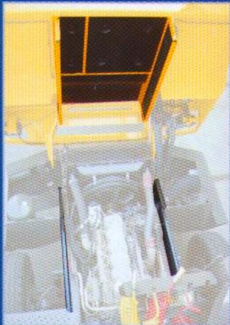
Standard feature: sound insulation material to ensure low noise levels.
