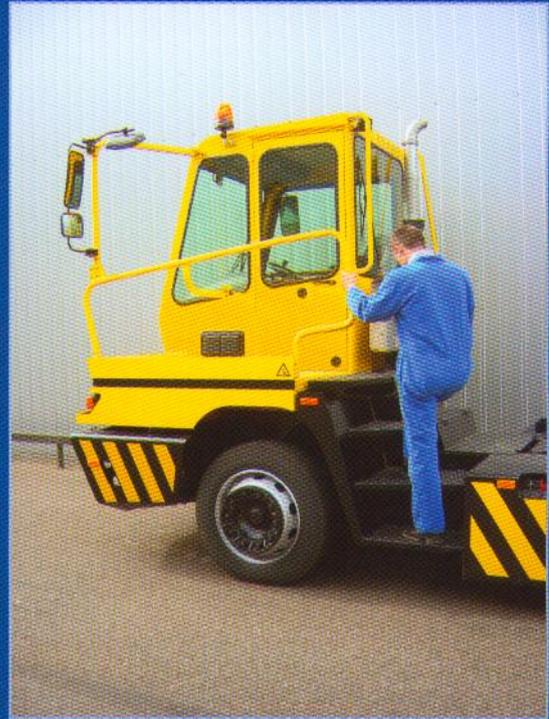
Standard feature: inboard door offers safe and easy cab access from either side of the tractor.
