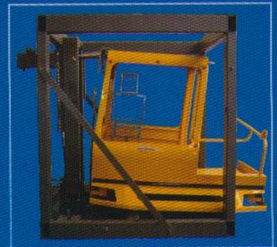
Strong, all steel cab structure (fully Fops & Rops tested), ensures maximum driver protection.
