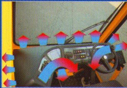
Cabin heating and (optional) cooling system with air supply to all directions
